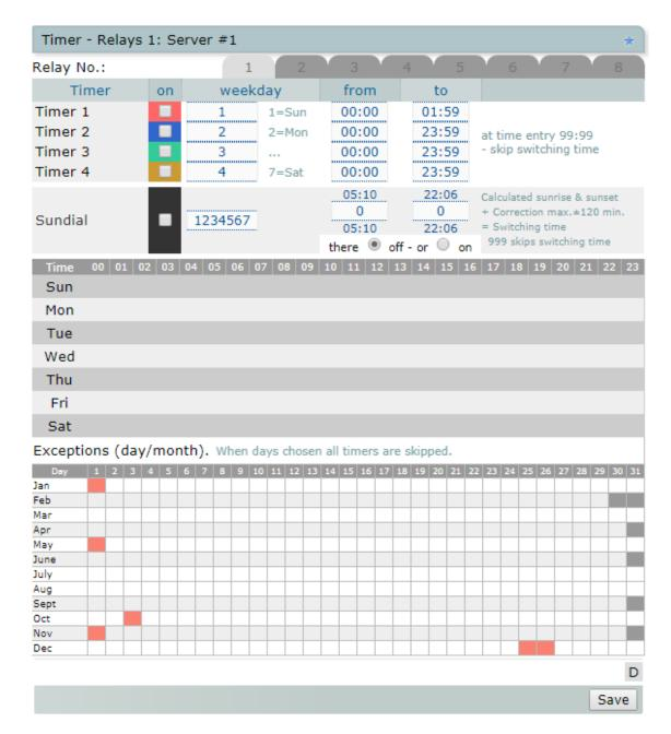
Sundial: The ,from' -'to' times are calculated automatically (2:00 AM) according to the information in the Time section. With: "In time off or on", it can be determined whether the relay should be switched: Is selected "In time off" = switched on at night - switched off during the day.
