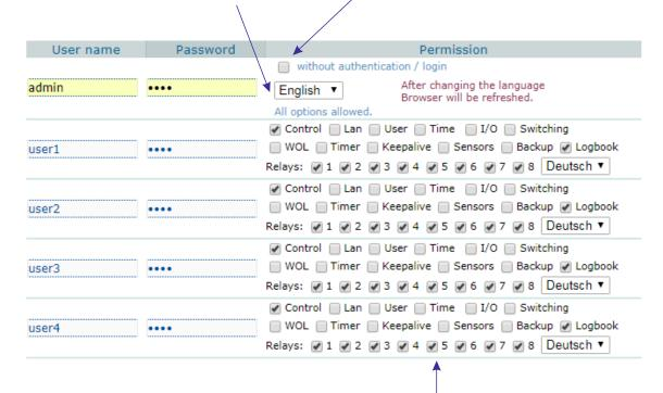
Relays/sockets can be disabled for users and displayed as inactive (as locked in Settings/Switching).
